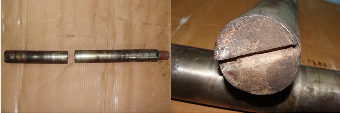
Figure 2. Fatigue failure of the axle.
