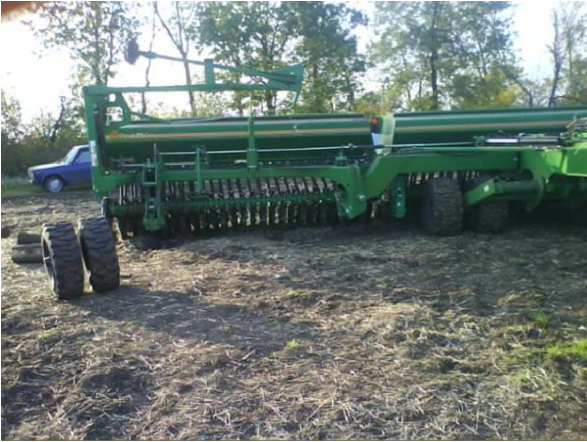
Figure 1. Grain drill, Note that the left side wheels are no longer attached to the grain drill due to an axle failure.
