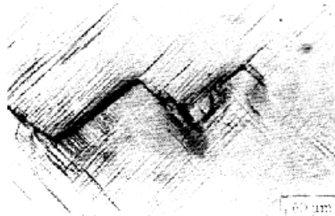
Stage I crack is strongly affected by slip characteristics, microstructure dimensions, stress level, extent of near tip plasticity
